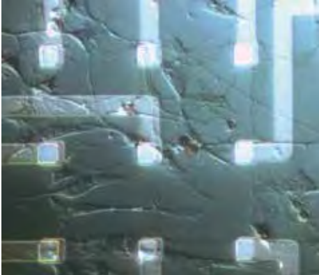
Symbol of the ETH's trend toward biology: neuronal networks connect on a microelectronic chip. Andreas Hierlemann, Institute for Quantum Electronics, 2005.
