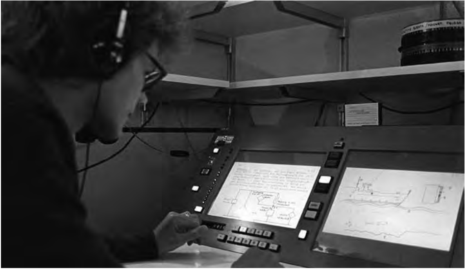
The desktop-computer-based, audiovisual, interactive PLANETH teaching system was developed and introduced at the ETH in the second half of the 1970s.
