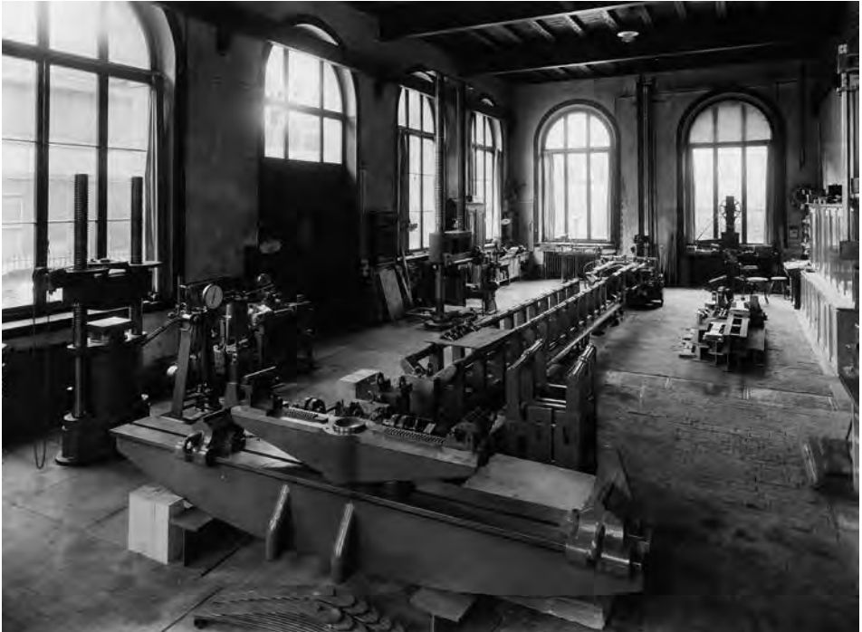
Werder's universal testing machine represented a milestone in experimental engineering science. The photograph, from 1892, shows the machine inside the Federal Materials Testing Institute.
